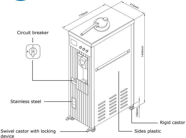
The L 07 HW water cooled unit must be connected to a  $\frac{1}{2}$ " water supply, minimum pressure 1.0 bar, highest pressure 6.0 bar.  $\frac{1}{2}$ " unpressurised water outlet. Water hoses used for connection must be approved for 15 bar operation.
